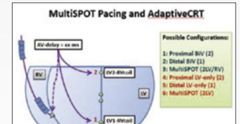
Advanced pacemakers that provide cardiac resynchronization therapy are small computers with the ability to sense and stimulate the heart using advanced patterns. Initial results using adaptive pacing in multiple locations are promising to further improve the effect of such implantable devices.
