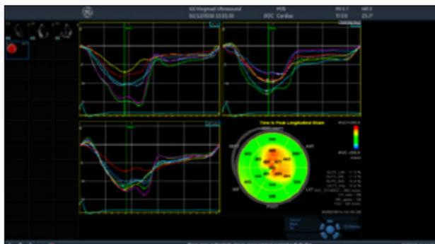
**Peak Strain Dispersion** is the GE marketing name for Mechanical Dispersion. This is a risk marker for sudden cardiac death and is computed automatically from a speckle tracking analysis. The feature is available in GE ultrasound scanners and the EchoPAC analysis station.
